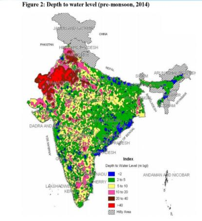
>Availability of groundwater in the northwestern region of the country is at very low levels **>**Significant pockets across the country where the depth of the water level is more than 10 meters. >In areas where water level is below 10 meters, sophisticated equipment is required to extract <u>it</u>
