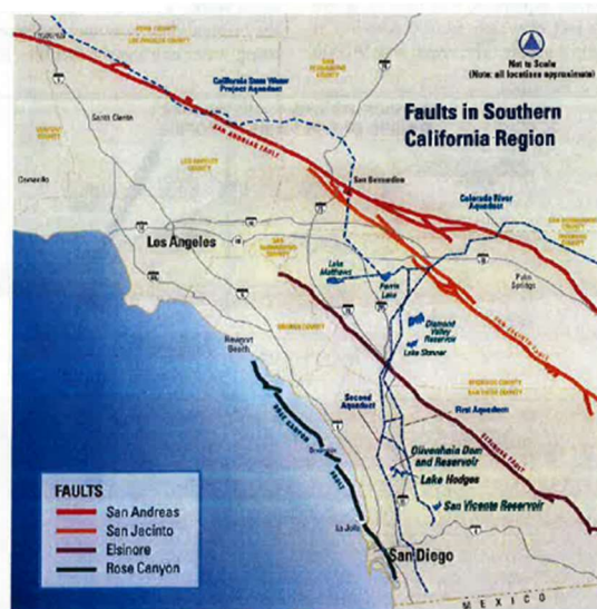
Figure 3. Water supply aqueducts cross major faults in Southern California
